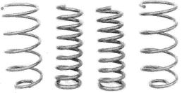
Compared to new factory springs, H-O springs lower the average car about 1½ inches in front and ½ inch in back—enough to lower the CG to improve cornering while maintaining enough travel to avoid bottoming out on rough roads and permit carrying heavy loads.
